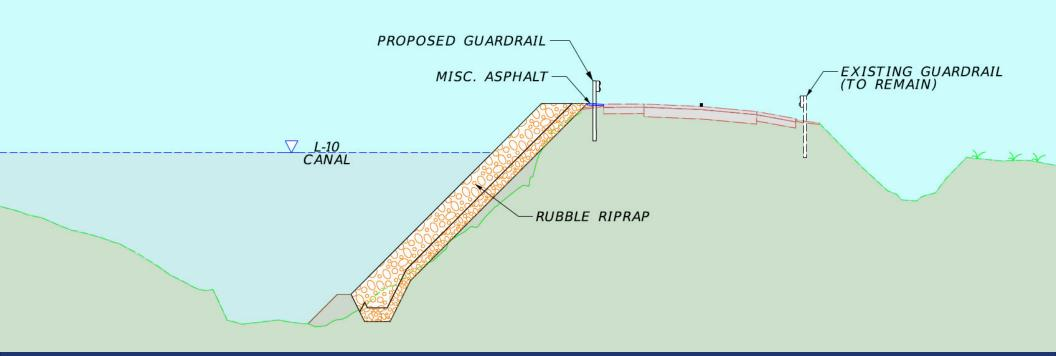
Typical section will be applied from West Main Street to north of the US Sugar railroad crossing, guardrail will be replaced, and damaged embankment sections will be stabilized and repaired using rubble riprap that matches the existing slope protection.
