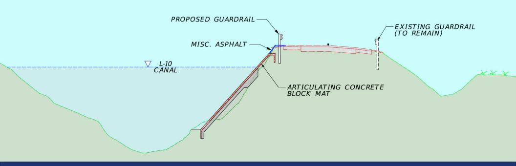
Typical section will be applied from the US Sugar railroad crossing to south of Hatton Highway, existing guardrail will be replaced along damaged embankment sections to be stabilized and repaired using articulated concrete block mats matching the existing slope protection.
